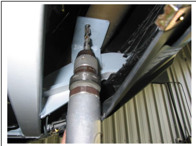
Figure 17 – Shown drilling cross member on passenger side
